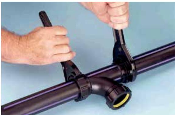
**NOTE:** Always tighten the nuts as work progresses. They should not be left until the job is completed. When installing a Vulcathene chemical drainage system the Vulcathene grooving tools and spanners must be used to ensure joint integrity.
