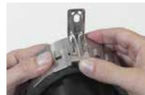
Ensure the correct number of brackets are always used and the two ends of the strip always have a connecting bracket.
