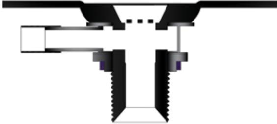
The illustration above shows the slotted version of the 504 waste assembly used in conjunction with the 509 overflow assembly. The waste, overflow collar and gaskets should all be set with a suitable sealant.
