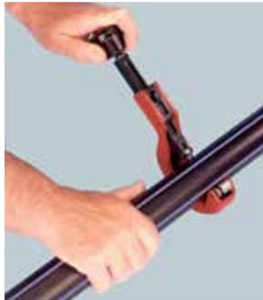
To achieve full joint integrity, it is essential that a groove is cut around the pipe with the appropriate grooving tool, into which the tongued olive will be located.
