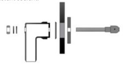
The below illustration shows a 509 overflow assembly with flexible hose to connect to the waste. The overflow bend and face-plate should be set with a suitable sealant.
