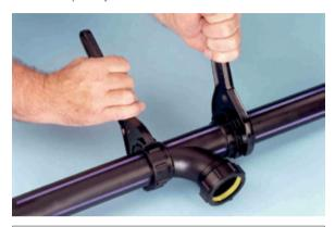
**NOTE:** Always tighten the nuts as work progresses. They should not be left until the job is completed. When installing a Vulcathene chemical drainage system it is imperative that Vulcathene grooving tools and spanners must be used to ensure joint integrity.
