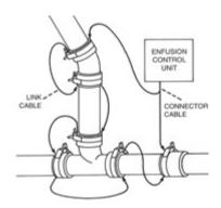
**Step 7** - Press the start button to begin the welding process. The enfusion control unit will display the temperature and the welding time.
