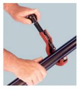
or burr on the pipe). The pipe must be square. If a saw is used, it is essential that all burrs and loose material are removed.
