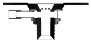
The illustration below shows the slotted version of the 504 waste assembly used in conjunction with the 509 overflow assembly. The waste, overflow collar and gaskets should all be set with a suitable sealant.
