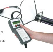
Vulcathene enfusion fittings incorporate moulded socket ends with an integral resistance wire in place. Jointing is completed by energizing the resistance wire via a dedicated enfusion control unit.
