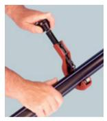
or burr on the pipe). The pipe must be square. If a saw is used, it is essential that all burrs and loose material are removed.
