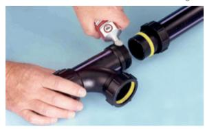
Loosely assemble the joint and proceed to hand tighten each nut. Using two Vulcathene spanners. The joint should then be tightened further to its full thread capacity.
